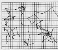
Perrin (1913) three colloidal particles, positions joined by straight lines
