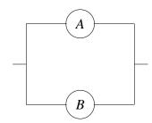
At risk of some confusion, we use the *letters A* and *B* for the *events* 'component *A* works' and 'component *B* works' respectively. Let *Y* be the event that current flows. Now, current flows if *either A* is working *or B* is working, so  $Y = A \cup B$ . Therefore
