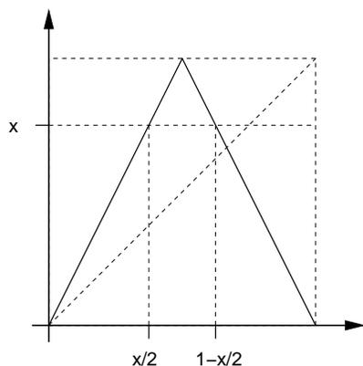
$$\begin{aligned} T(x) &= 1 - |1 - 2x| \\ T^{-1}(x) &= \left\{ \frac{x}{2}, 1 - \frac{x}{2} \right\} \\ |T'(x)| &= 2. \end{aligned}$$
