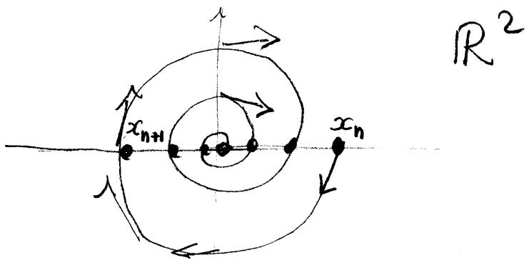
In the above example, the transit time between intersection of an orbit with the  $x$ -axis need not be unity, in which case the index  $n$  simply counts such intersection. This construct is called a surface of section.
