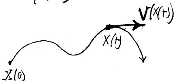
It can be proved that the vector  $V(X(t))$  is tangent to the curve at  $X(t)$ . Such a curve is called the orbit through  $X_0$ .
