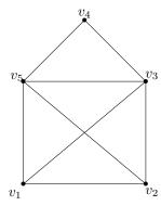
Then  $R = v_1v_2v_3v_4v_5v_1v_3v_5v_2$  is an Euler trail for G, but G has no Euler tour.
