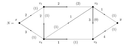
The flow along an arc is given by the number in brackets and its capacity by the number not in brackets. We have  $val(f) = f^+(x) - f^-(x) = (1+1) - 0 = 2$ .
