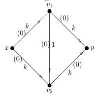
The capacities of the arcs  $xv_1, v_1y, xv_2, v_2y$  are all equal to k where k is a large positive integer. Suppose we run the Ford-Fulkerson algorithm on N. We start with the 'zero flow'  $f_1$ , by putting  $f_1(e) = 0$  for all  $e \in A(N)$ . The first iteration of the algorithm could find the  $f_1$ -unsaturated xy-path  $P_1 = xv_1v_2y$ . The maximum amount of flow we can send along this path is  $s(P_1) = 1$ . This gives rise to the new xy-flow  $f_2$  shown below which has value 1.
