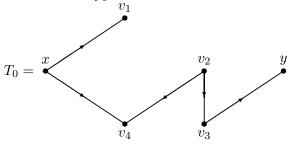
**Step 2** T contains y. Use the  $f_1$ -unsaturated xy-path  $P = xv_4v_2v_3y$  in T to define a new flow  $f_2$  with  $val(f_2) = val(f_1) + s(P) = val(f_1) + 1$ .
