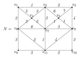
An implementation of Dijkstra's algorithm starting at  $v_1$  produces the following tree  $T_4$  at the end of the fourth iteration:  $V(T_4) = \{v_1, v_2, v_3, v_6\}$  and  $E(T_4) = \{v_1v_2, v_2v_3, v_1v_6\}$ . It also gives the vertex labels shown in the following table.
