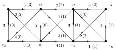
The numbers in brackets define an xy-flow  $f_1$  in N. The numbers not in brackets define the capacities of the arcs of N.
