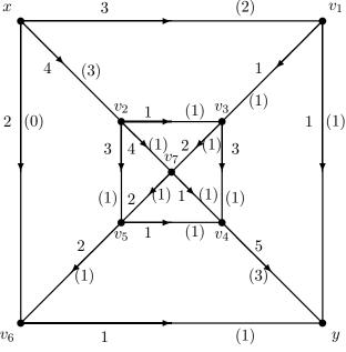
Numbers in brackets denote the flow  $f_1(e)$  along each arc e, numbers not in brackets denote the capacity c(e) of each arc e.
