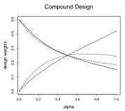
Support points and the weights of the compound optimum design for  $\lambda_1^o=\lambda_2^o=1$  as a function of  $\alpha$
